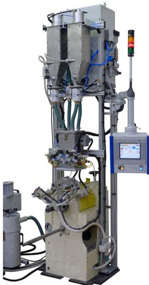
Old Sprimag machine equipped with Frei-Powder system including control and filter unit for a production capacity of 150 cpm.
