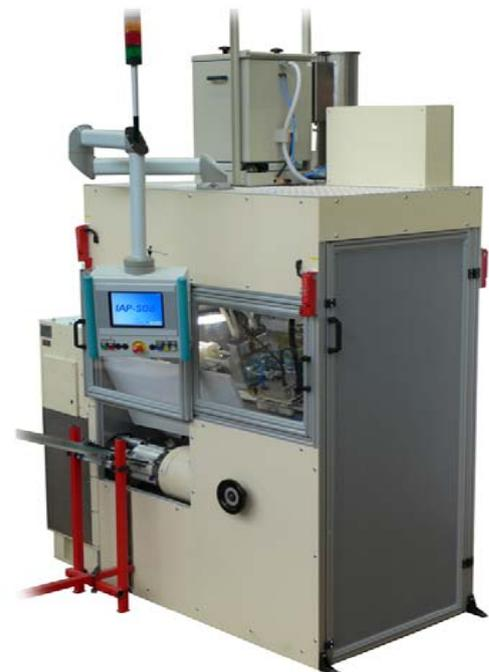
Frei IAP-S06 powder coating system mounted on an old wet lacquer spraying machine for tubes with membrane. Special: The cam disc drive has been replaced by servos allowing an even more precise powder particle distribution.
