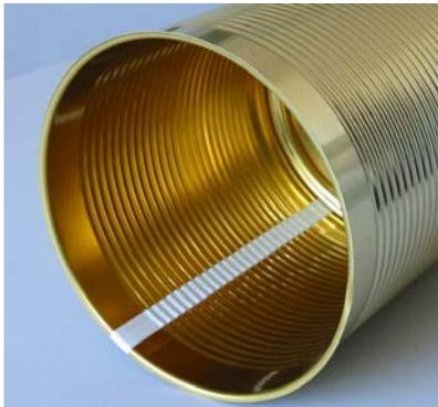
Powder has to be used to obtain an optimized and pore-free seam that withstands the flanging, necking and beading processes as well as the aggressiveness of the filled products.
