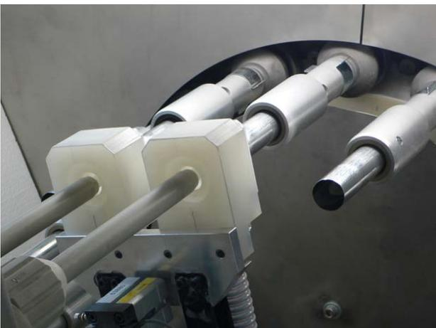
conveyor on which the rotating cans travel in horizontal position past a group of parallel powder guns. The guns move along with the cans or tubes as they reciprocate in and out
