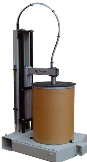
injector system for precise feed rating makes it possible for the operator to determine the required quantity of powder fast and simple.
