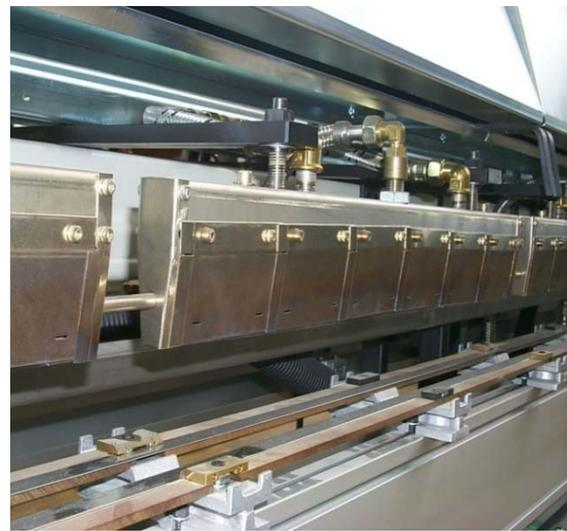
*Frei AG curing unit, model ECM equipped with the original „first generation ECO burners“. These burners were the first ones in the market that guaranteed lowest NOx and CO exhaust emissions.*
