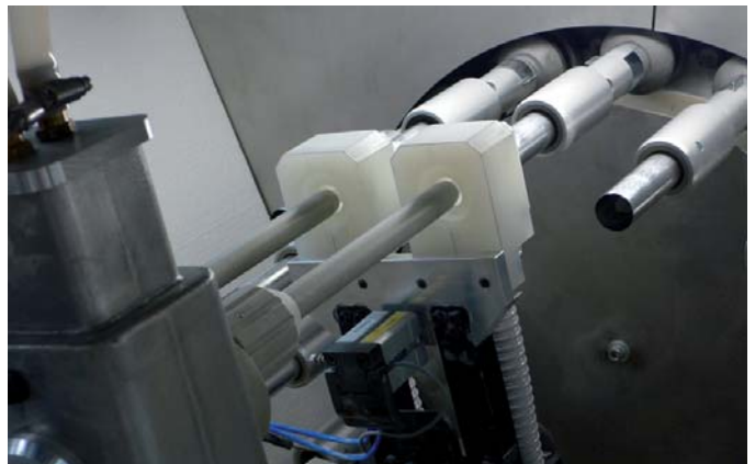
Integrated additional exhaust and cleaning modules guarantee an absolute dust-free environment for the cans and the whole machine
